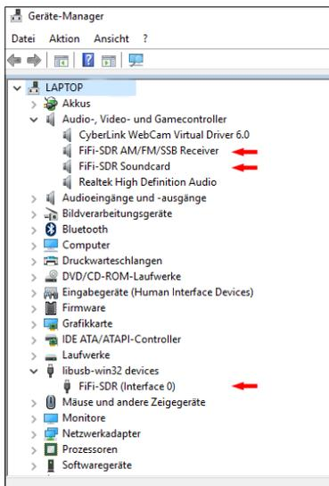
*The FiFi-SDR correctly displayed in the device-manager after successful driver installation.*
