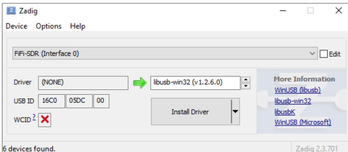
6. In the selection box indicated by the green arrow select the driver, *libusb-win32* and then click *Install Driver*. Both the other FiFi-SDR interfaces (*AM/FM/SSB-Receiver* and *FiFi-Soundcard*) use the *libusbaudio* so no further intervention is required.
